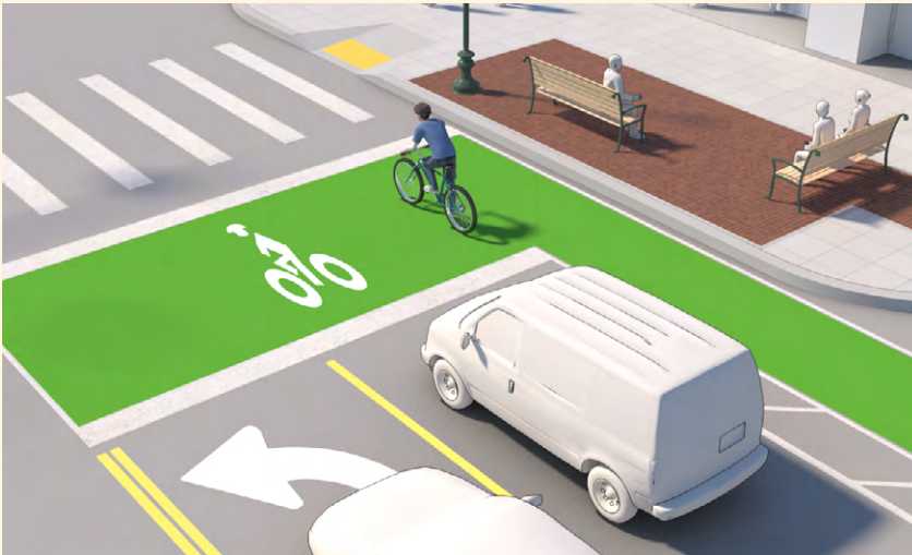
Illustration of a bike box, from the NJDOT Complete Streets Design Guide, used to mitigate conflicts between bicycle and motor vehicle traffic at signalized intersections and improve the visibility of bicyclists.
