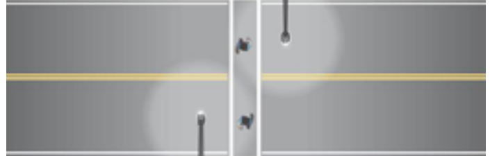
Figure 9. Design for mid-block crossing lighting layout (Courtesy of VTC).
