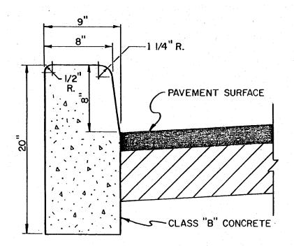
NOTE: TRANSVERSE JOINTS I/2" WIDE SHALL BE INSTALLED 10'-0" APART & SHALL BE FILLED WITH PREFORMED BITUMINOUS JOINT FILLER AASHO DESIGNATION M 213 RECESSED I/4" FROM TOP AND FACE. DEPRESSED CURB AT DRIVEWAYS PER 605.02, NJDOT STD SPEC. FOR ROAD AND BRIDGE CONSTRUCTION, 1989.
