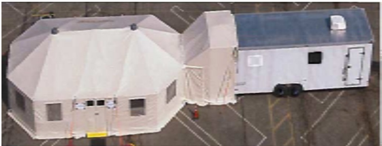
One module of the Western Shelter System is shown connected to one of the two support trailers.
